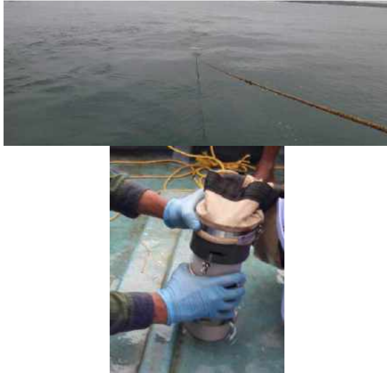
Plate: 2.4: Towing of bongo net in surface waters for zooplankton and removal of bucket from bongo net to collect zooplankton sample
