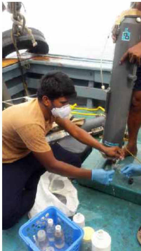
Plate 2.3: Collection of waters samples from Niskin sampler
